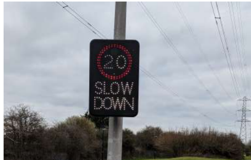
Temporary vehicle activated speed sign installed at the Maltlands earlier this year
